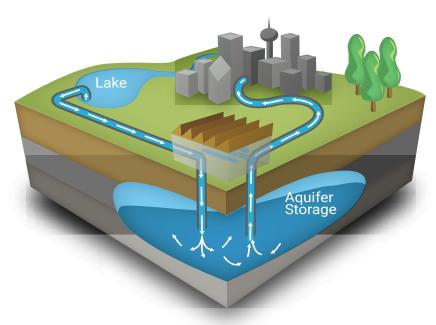
During times of plenty, extra water can be stored underground so that it can be used during drought or other similar circumstances. The supply source for ASR can be surface water from rivers, treated wastewater, groundwater from other aquifers, or even captured stormwater runoff.
